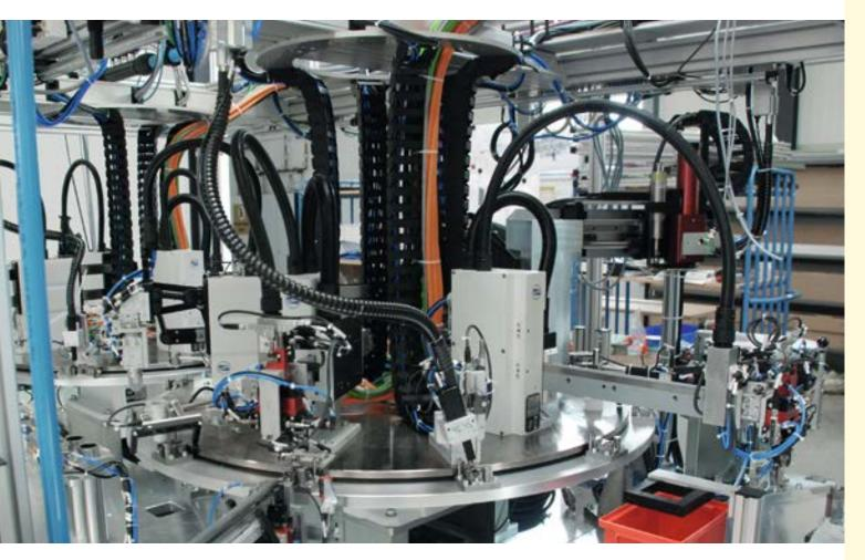
Whether HP 140 or HP 70: The Pick & Place from WEISS works with two linear axes and therefore profit from all advantages of a direct drive: rapid dynamic performance, free user-programmability, minimal wear and highest precision. The HP overcomes limits of traditional pneumatic systems regarding variability, dynamic performance and efficiency.
