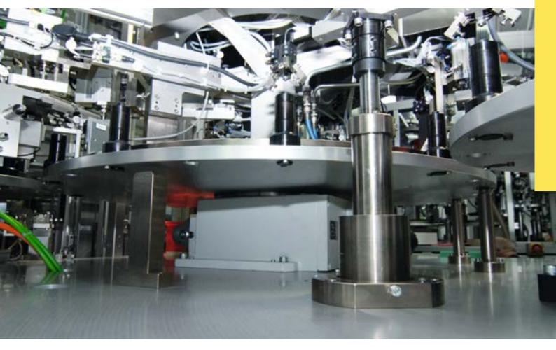
Custom machine for an automotive supplier. A user-programmable NC 320 represents the heart of the system. It brings the seal and springs together and forwards the components to the other tables.
