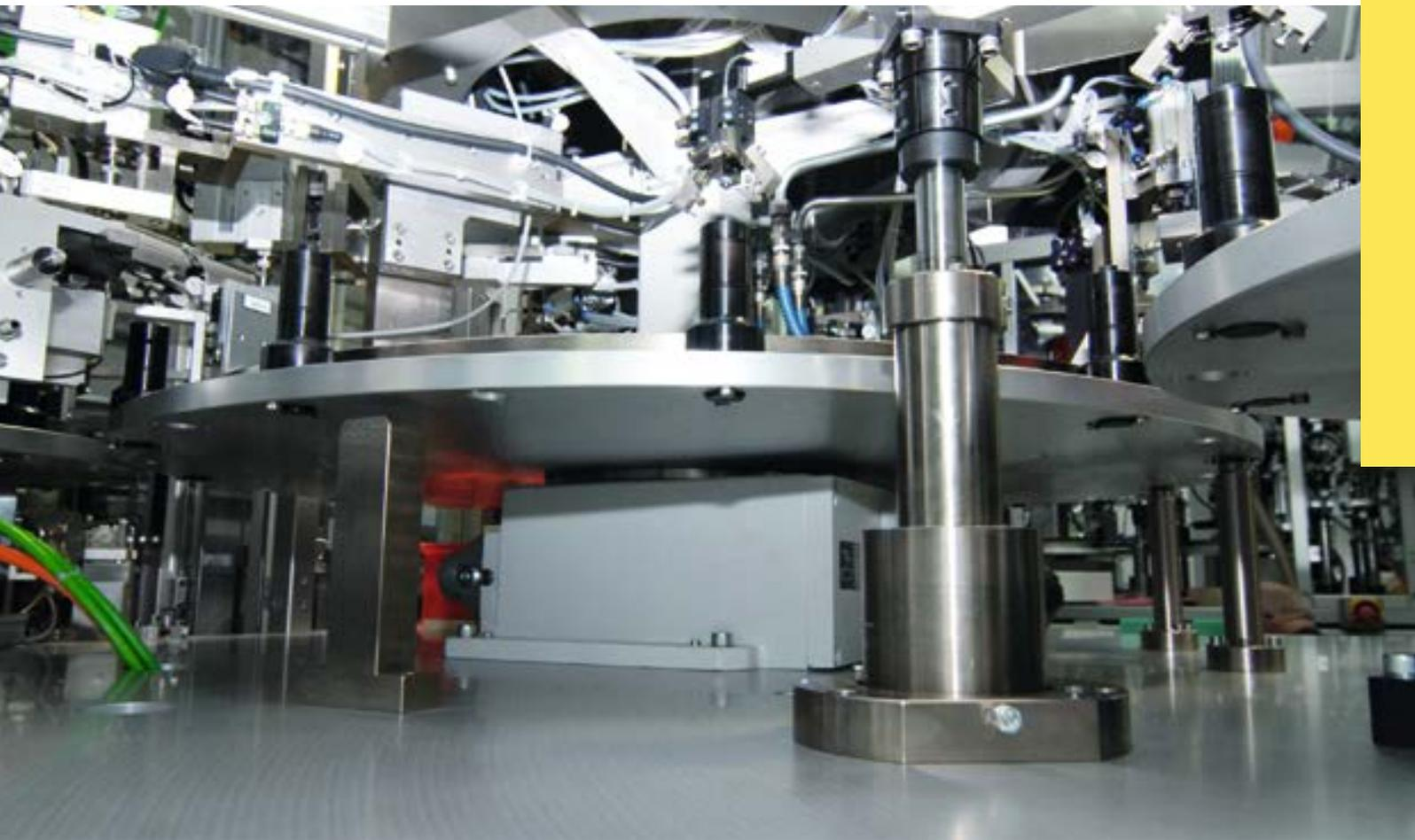
Custom machine for an automotive supplier. A user-programmable NC320 represents the heart of the system. It brings the seal and springs together and forwards the components to the other tables.
