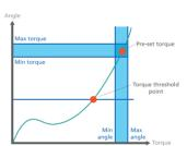
It's the most common mode. If the final torque and angle values are within the preset minimum and maximum values, the screw is tightened correctly and the controller will give an OK message.
