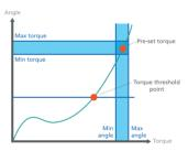
its the most common mode. If the final torque and angle values are within the preset minimum and maximum values, the screw is tightened correctly and the controller will give an OK message.
