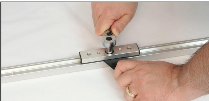
**Fig. 2: Fit up adjustment**
