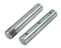
To get the best performance from your Pacific bearings we suggest the use of Hepco's linear shafting, hardened and ground to RC60 (other options available). Surface finish. .20-.40µm.
