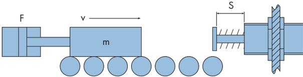
$$E_1 = \frac{m \times v^2}{2} = \frac{16 \times 1.4^2}{2} = 15.7 \text{ Nm}$$
