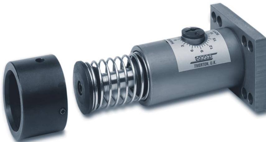
**Hepco SH Shock Absorbers will match the speed and mass of the moving object and bring it to rest with no shock - the energy will simply be dissipated, mostly as heat. They also out-perform cylinder cushioning or dashpots, dissipating the energy at a uniform rate, thus enabling far faster stopping times to be achieved. The range offers adjustable and non-adjustable full threaded metric type shock absorbers together with fixed flange adjustable type up to 28mm bore size.**
