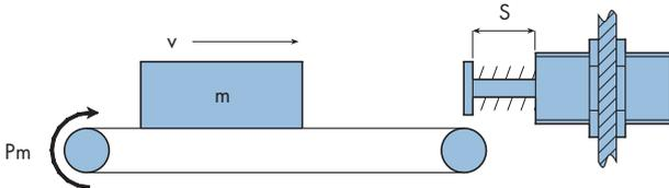
$$E_1 = \frac{m \times v^2}{2} = \frac{50 \times 0.9^2}{2} = 20.25 \text{ Nm}$$
