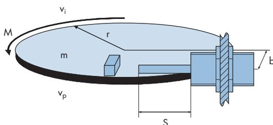
$$E_1 = \frac{m \times v_p^2}{4} = \frac{100 \times 0.8^2}{4} = 16 \text{ Nm}$$
