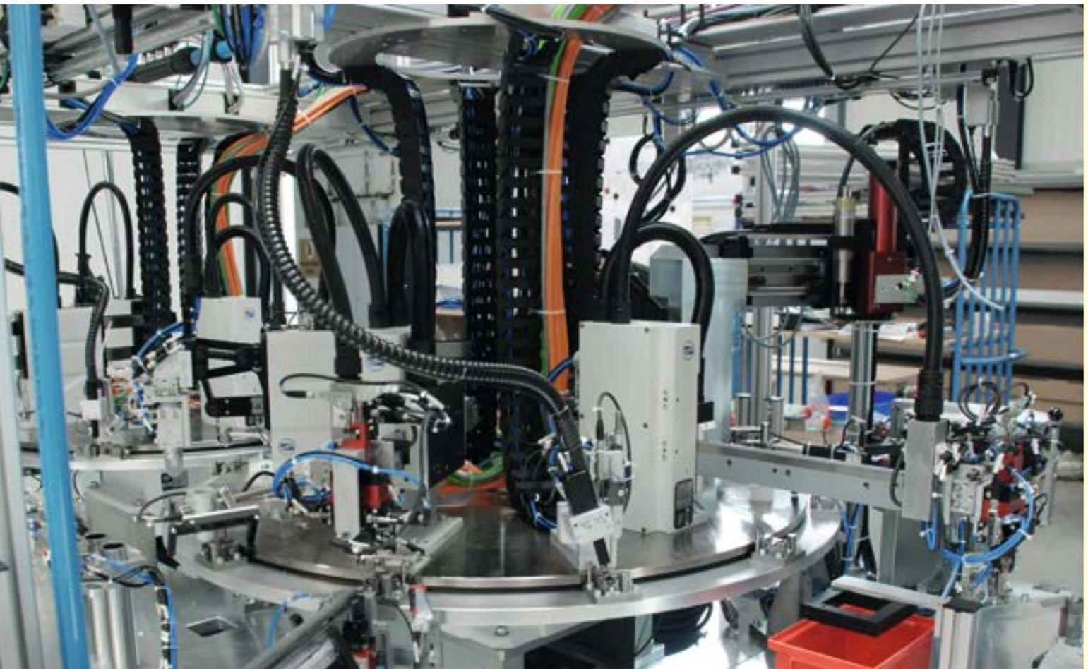
Whether HP 140 or HP 70: The Pick & Place from WEISS works with two linear axes and therefore profit from all advantages of a direct drive: rapid dynamic performance, free user-programmability, minimal wear and highest precision. The HP overcomes limits of traditional pneumatic systems regarding variability, dynamic performance and efficiency.
