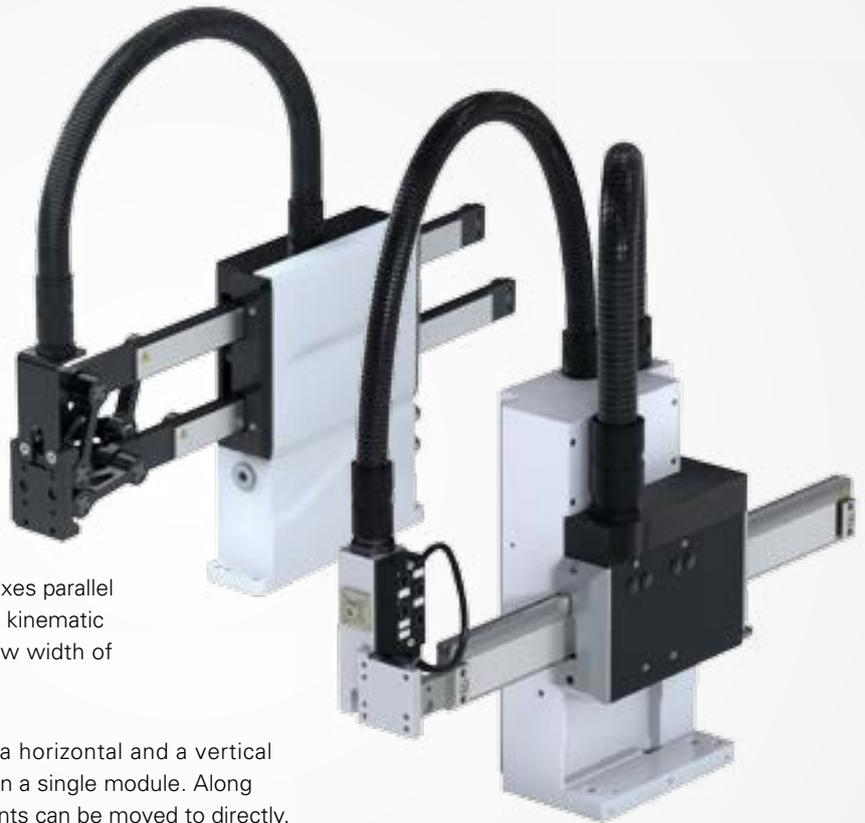
Pick & Place HP 70: two horizontal linear axes parallel on top of each other, connected through a kinematic unit. Because of the construction a narrow width of only 60 mm is possible.
