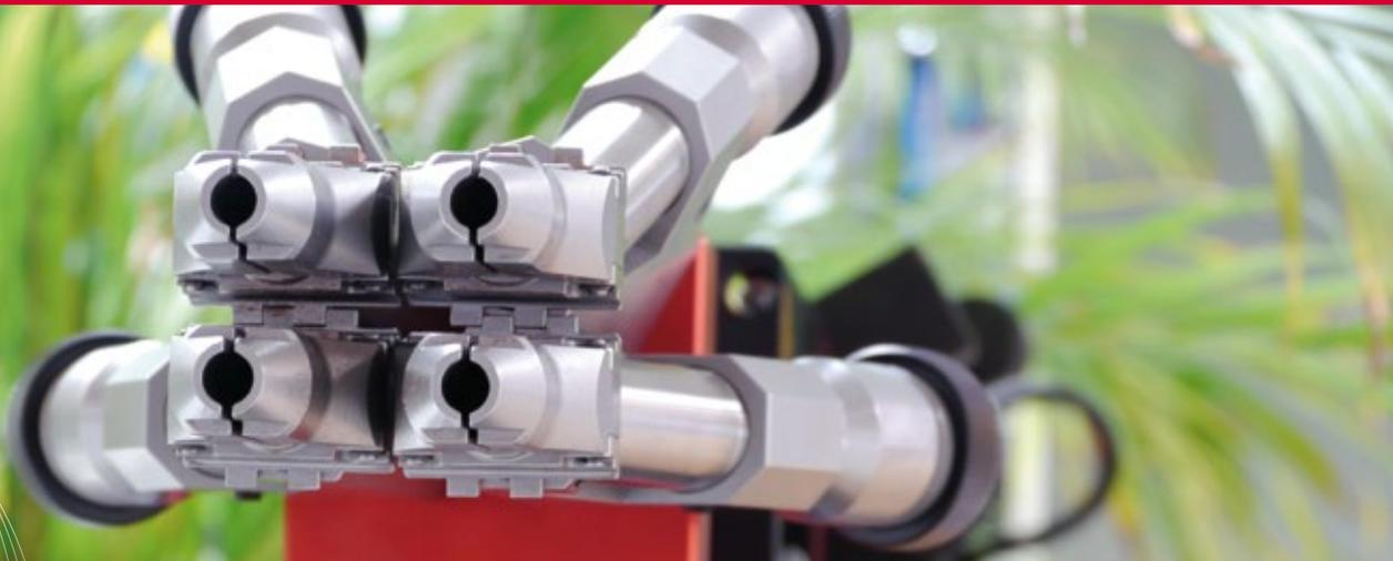
A multi-spindle machine is used when several fasteners (of the same or different type) have to be processed in one work piece within a short cycle time.
