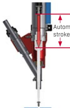
A pneumatic cylinder causes the screwdriving tool to travel to the screw. Screw is positioned in screwdriving location
