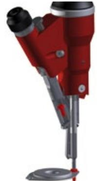
During the screwdriving process, the nose piece retracts upwardly away from the work piece without touching it.
