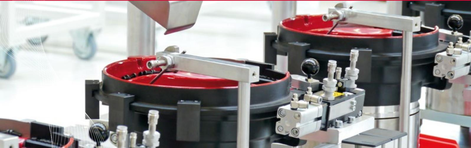
Due to the large variety of fastening elements and applications feed systems have to meet different requirements: screws with differing geometries as well as coated, micro-encapsulated and lubricated screws have to be sorted and fed correctly, short cycle times have to be achieved, they should be quiet in operation, avoid abrasion, etc. Thus, several types of feed systems based on different operating principles
