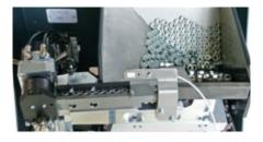
**Step feeder (STF):** suitable for all types of fastening elements, low in vibration
