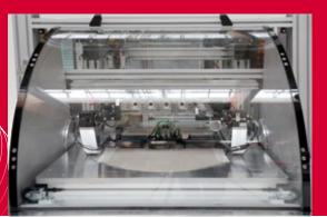
Due to a variety of individual applications assembly cells are available in different versions: with roller shutter, automatic sliding door or light curtain, with turntable or safety drawer to position the work piece, as well as with any possible add-on. Further operational steps can be integrated, such as lubricating, adhesive bonding, machining the work piece, scanning of bar codes or printing of labels, etc. Our modular assembly cell was developed in order to meet any possible requirement.
