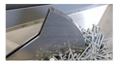
Segment feeder (SGF): particularly suitable for fasteners with sensitive surface, works without vibration
