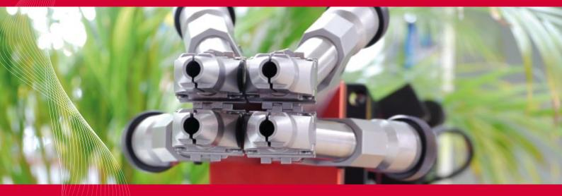
A multi-spindle machine is used when several fasteners (of the same or different type) have to be processed in one work piece within a short cycle time. Multi-spindle systems may be based on our standard models or newly developed according to the customer specification.
