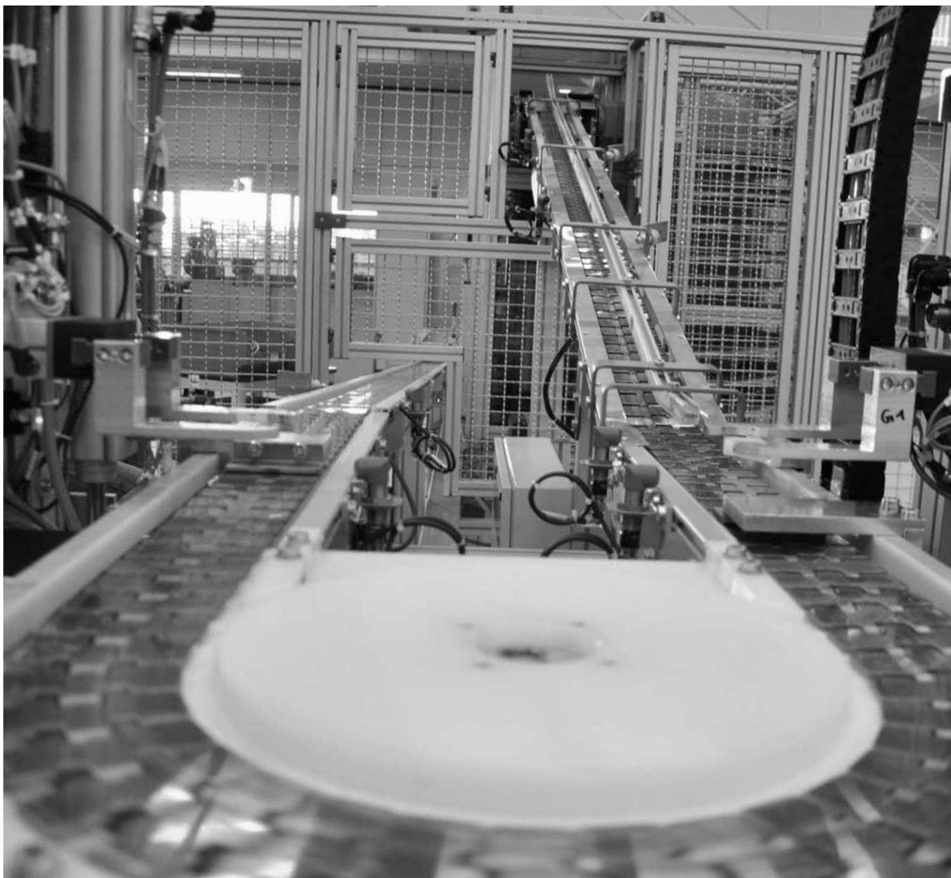
All chains are suitable for directly transporting the products or transporting the pallets.
