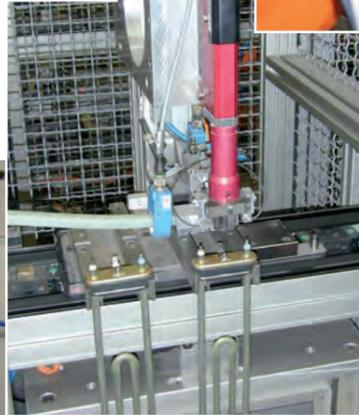
Fitting nuts to heating
