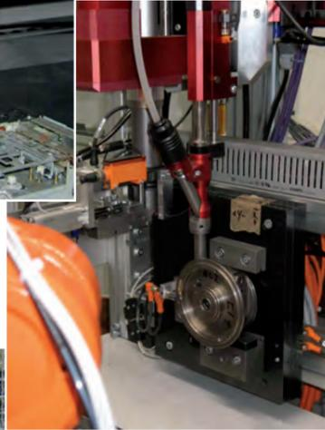
Fitting studs to a turbo-
