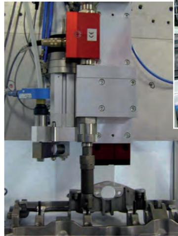
Fitting studs to cylinder heads
