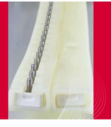
sluice or the escapement, it is ejected and fed to the screwdriver head with the correct orientation for processing.
